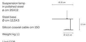
1 led COB 14W - 350mA 2900 Lm emitted 3000°K - CRI 85 Phase cut dimmable power supply included
