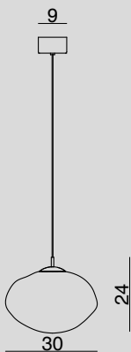
GIG1653.1L SOSPENSIONE A ROSONE / HANGING LAMP WITH CANOPY Glass 1 x Ø 30 cm - Cable 200 cm 1 x LED 8,4 W DIMM
